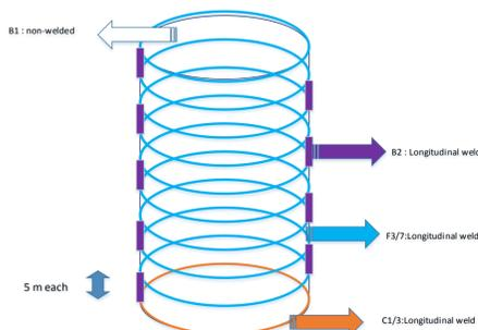
Figure 3: showing applications of different welds to the model.
