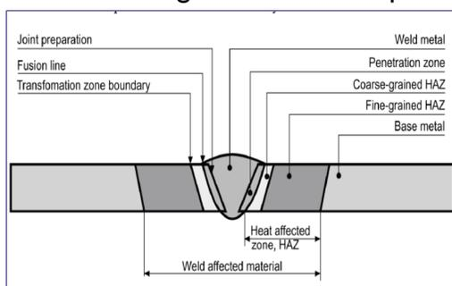
Welded joint and HAZ [4]
