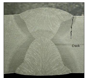
Fatigue Crack in Butt weld (adapted[5])
