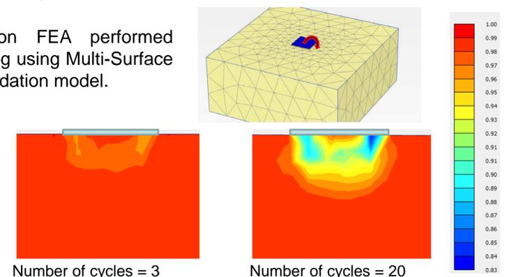
Figure 4.2 Shallow foundation cyclic degradation example
