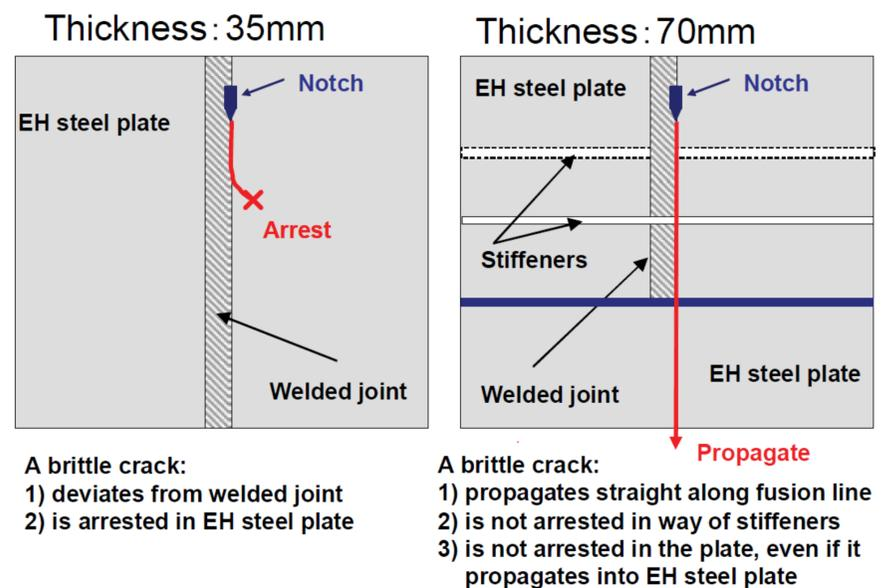
Figure 2. Effect of increased plate thickness of crack arrest behaviour in EH shipbuilding structural steels. (Sugimoto, 2010)
