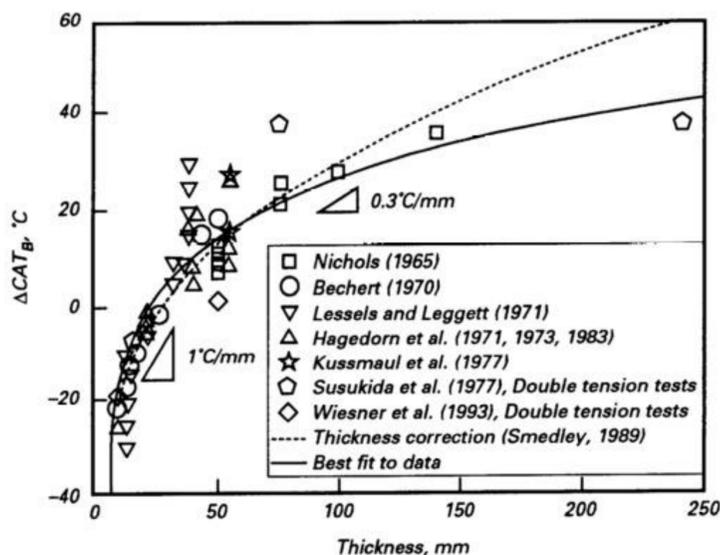
Figure 1. Change in CAT compared to that of a plate with 25mm thickness. A large amount of scatter is shown in samples above 50mm thickness. (Wiesner, 1995)
