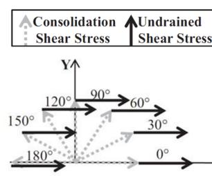
Stress path on soil sample showing first consolidation shear stress followed by undrained shear stress
