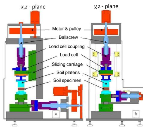
Schematic of VDDCSS operation mechanism
