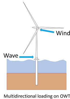
Multidirectional cyclic loading caused by wind and wave loads
