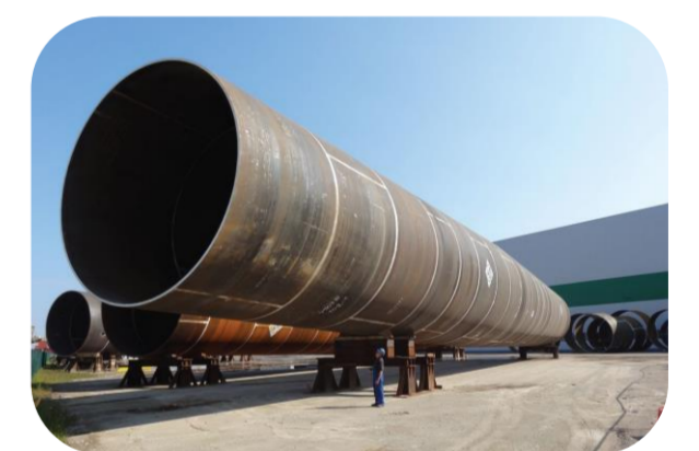
6. Monopile is ready to go offshore
