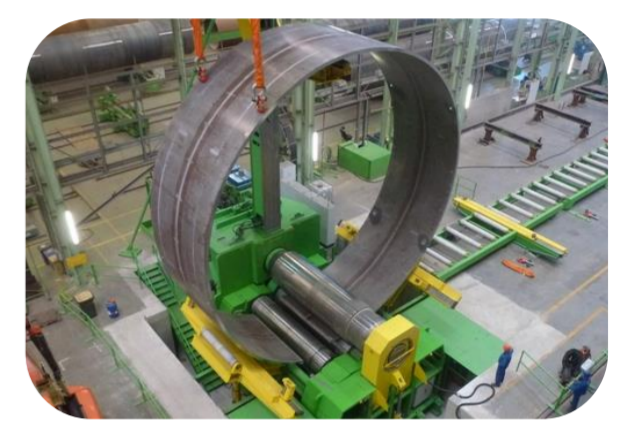
2. S355 hot rolled plates undergo cold rolling to form cans
