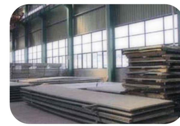
1. Plates of S355 are hot rolled
