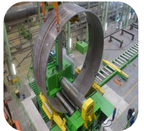
2. S355 hot rolled plates undergo cold rolling to form cans
