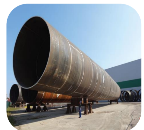
6. Monopile is ready to go offshore
