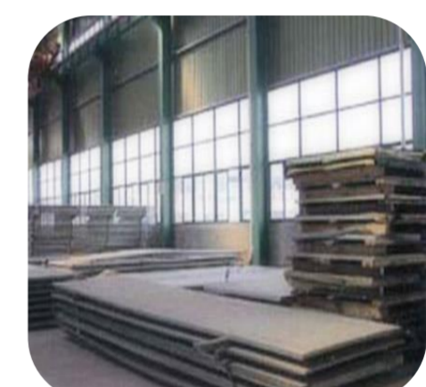
1. Plates of S355 are hot rolled
