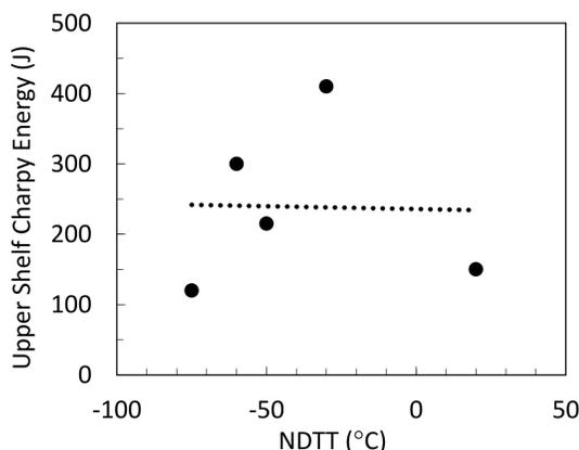
Figure 2: initiation fracture toughness from Charpy tests vs crack arrest toughness from Pellini tests (NDTT)
