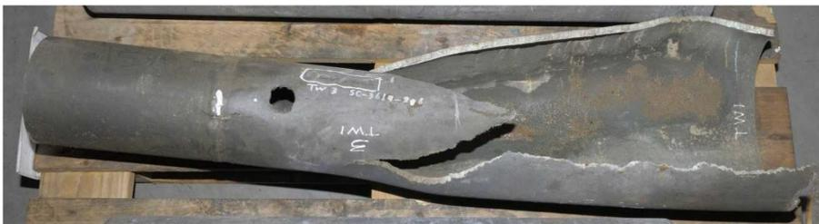
Figure 1: result of a brittle crack's failure to arrest in a pipeline can cause catastrophic failure.
