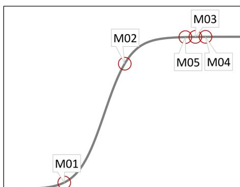
Figure 3: schematic representing where the NDTT lies on the Charpy curve for each material.
