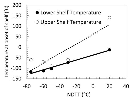
Figure 4: temperature of the onset of the shelf (upper/lower) vs NDTT
