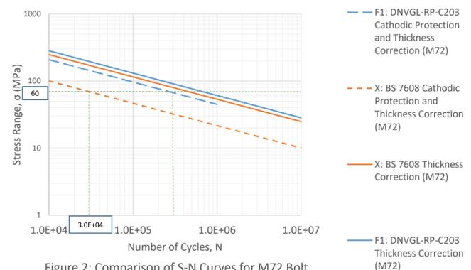
Figure 2: Comparison of S-N Curves for M72 Bolt in Air with M72 Bolt with Cathodic Protection
